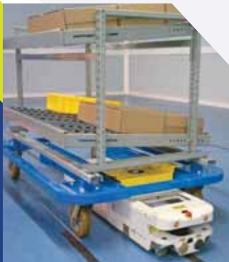
An Automated Vehicle delivers a SmartDolly cart with a Gravity Flowrack.
