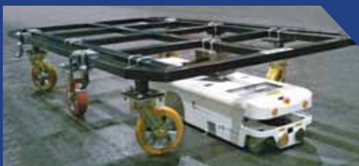
Small, powerful and smart: Automated Guided Vehicles are mobile robotics that "tunnel" underneath the MMPEX SmartDolly to propel it along its magnetic tape paths.
