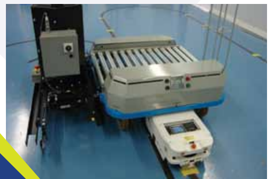
A Guided Vehicle delivers SmartDolly carts to a MMPEX Rapid Dolly Exchange Rotator. The Rotator can exchange an empty dolly with a loaded one. Excellent for supplying assembly lines in space-restricted applications.
