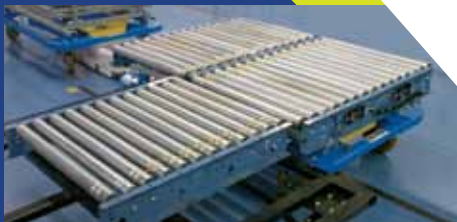
A MMPEX SmartDolly cart with installed Conveyor Flow being delivered by an Automated Vehicle.
