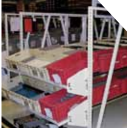
Storage Flow Systems — comprised of bins, totes and containers — can be serviced either robotically or manually.
